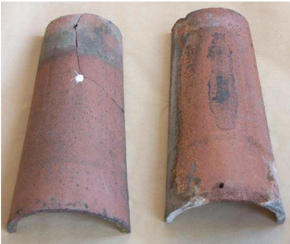
Historic cover tile on left. Historic pan tile, shown upside-down, on right. Both tiles are identical in shape, but the attachment hole is at the narrow (top) end of the cover tile and the wide (bottom) end of the pan tile. Note tar and mortar stains on the pan tile. These two tiles differ somewhat in texture and color, but further evaluation is needed to determine if this variation is typical of all the tiles.
