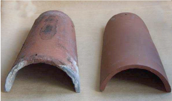
Historic tile on left. New, less curved tile on right. New tile is also thinner and more uniform in texture.
